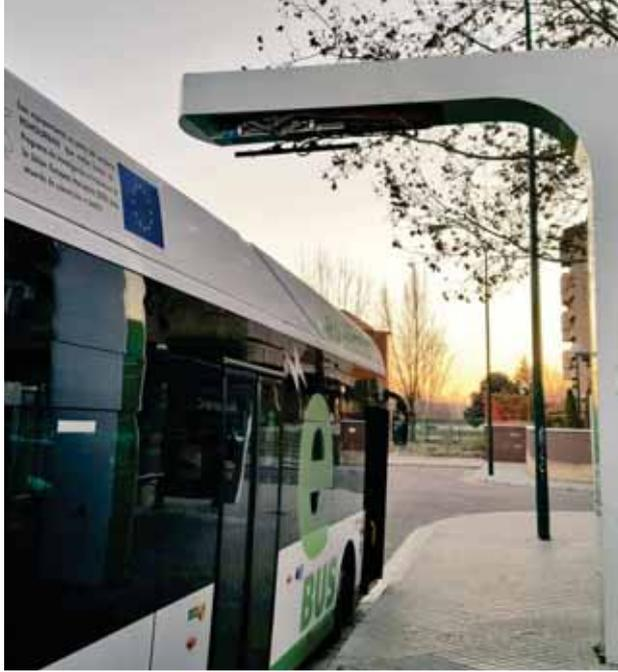
The buses then automatically enter their fully-electric mode upon arrival in the city centre, covering 70 per cent of the line in this mode (four kilometres out of the six-kilometre length of the line).
